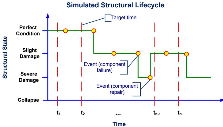
Figure 1: Using DES to generate a structural lifecycle
