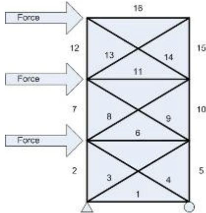
Figure 3: Statically indeterminate 16-member truss structure
