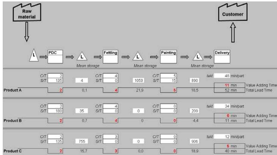
Figure 5: The VSM representation with the first 3 products shown.
