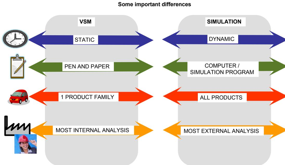
Figure 1: Some important differences between VSM and simulation.
