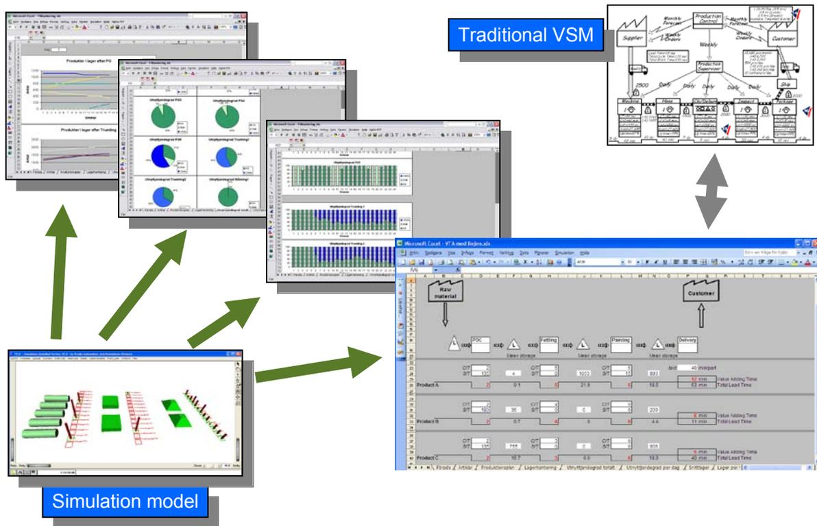
Figure 6: Simulation Based Value Stream Mapping (SBVSM)
