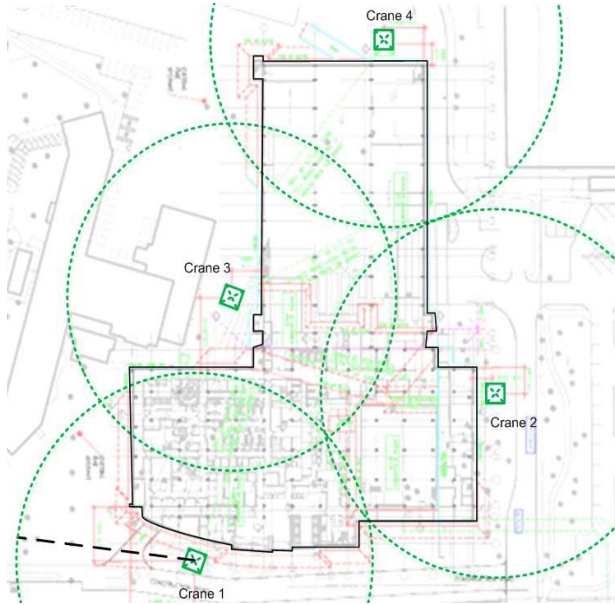
Figure 7: PCL construction site layout
