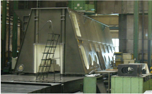
Figure 3: Ships engine crankcase – treatment operations(source: HCP)
