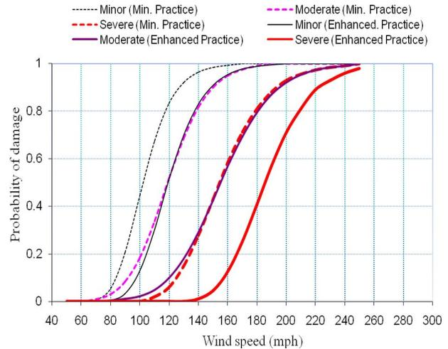
Figure 1: Probability of Hurricane Damage (Minimum and Enhanced Construction Practices)
