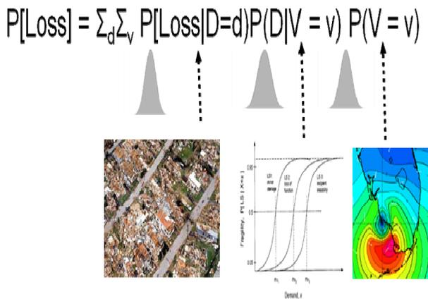
Figure 5: Regional hurricane loss estimation framework using fragility and virtual globe application to display storm track and observation information.
