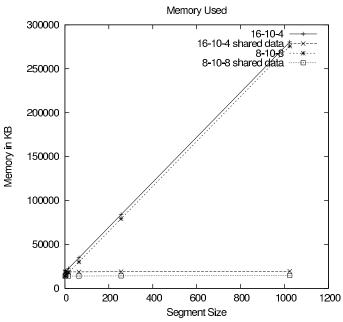
Figure 5: Memory required with respect to shared data segment size. One case is 8 multicast trees, 10 levels and 8 start events and the other case is 16 trees, 10 levels and 4 start events.
