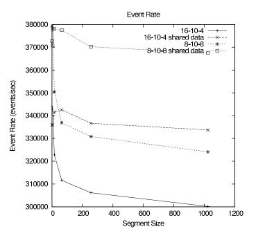
Figure 6: Event Rate with respect to shared data segment size. One case is 8 multicast trees, 10 levels and 8 start events and the other case is 16 trees, 10 levels and 4 start events
