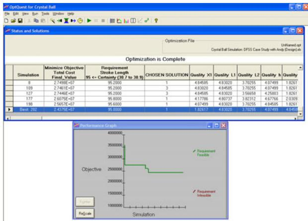
Figure 12: Minimization of Costs Subject to 95% in Specification Requirement
