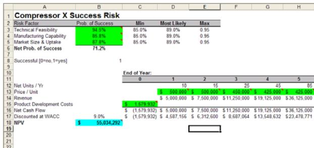
Figure 1: Compressor Feasibility Spreadsheet
