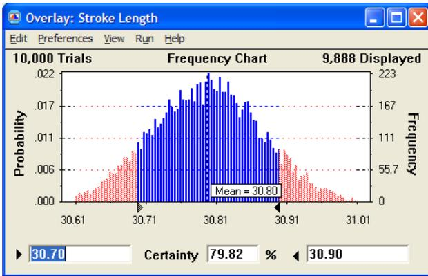
Figure 11: Certainty of Achieving Specification Limits on Stroke Length
