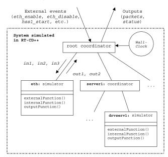
Figure 3: RT-CD++ Simulation Scheme
