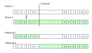
Figure 4: High Level Crossover Operator
