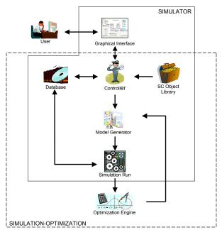
Figure 1: Simulator and Simulation-Optimization Modular Components
