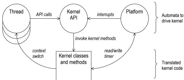
Figure 3: Structure of Kernel and Environment Models
