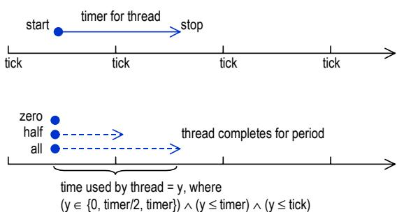
Figure 5: Original Timer Options for Elapsed Time When Thread Completes for Period
