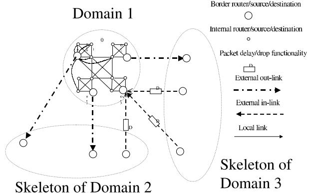
Figure 3: Domain Simulator Structure
