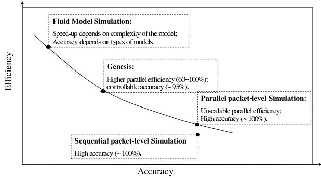
Figure 2: Simulation Efficiency vs. Accuracy
