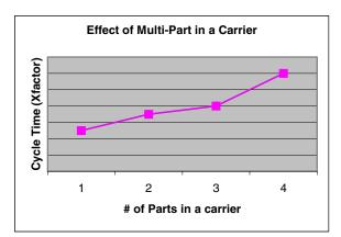
Figure 4: Effect of Multi-Parts in a Carrier
