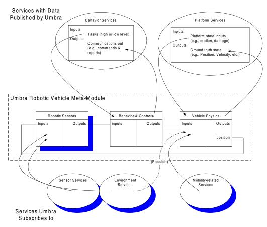
Figure 4: Conceptual Diagram Showing Umbra-to-HLA Integration for a Robot Vehicle
