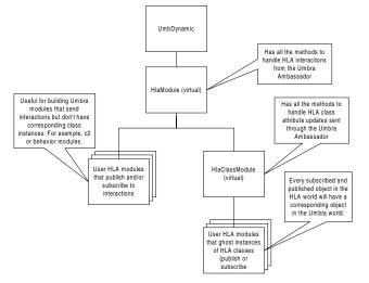
Figure 5: Typical Class Hierarchy for Application-Specific HLA Objects
