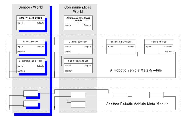
Figure 2: Umbra Robotic Vehicle Example Showing Relationship between Meta-Modules and Multiple Worlds. Simulation clock module and related ports and connectors are omitted.
