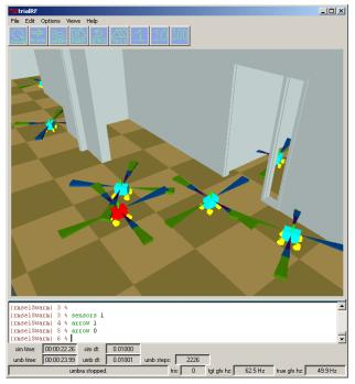
Figure 3: Umbra Simulation of Robots Collaboratively Exploring, with Sensor Response Regions Shown
