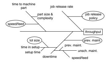
Figure 2: Cause-effect Diagram for the Machine Shop Study
