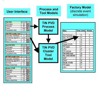
Figure 2: HSE Model Integration
