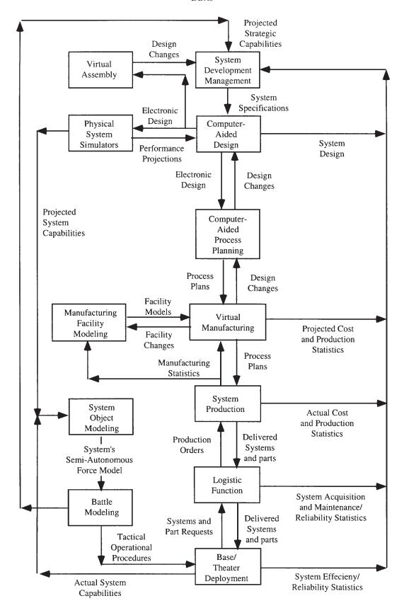
Figure 1: Schematic for the Overall System Acquisition Function
