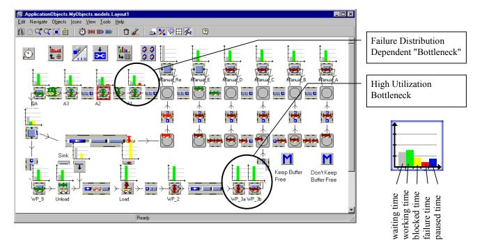
Figure 1: eM-Plant Model Showing Bottleneck Detection
