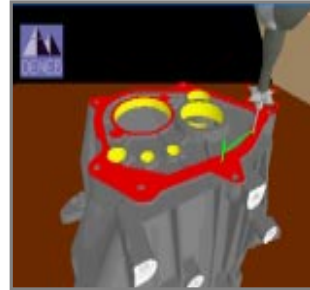
Figure 10: CMM Program Generation from CAD Data
