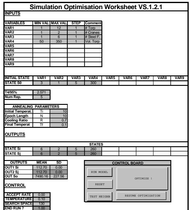
Figure 3: Front End of the Simulation Optimization Procedure (Excel Spreadsheet)
