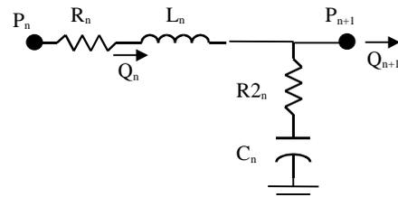
Figure 2. Electrical Circuit Model of Arterial Vessel (Snyder, Rideout)
