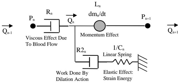
Figure 3. Visco-Elastic Mechanics Model of Arterial Vessel (O'Neil)
