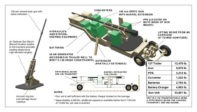
Figure 5: SPETC Gun Concept 3D Model
