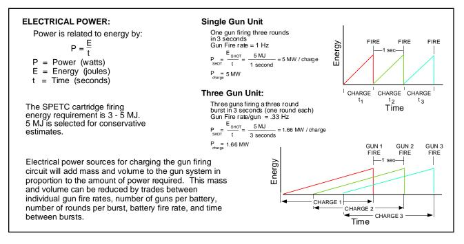
Figure 3: Preliminary Electrothermal Gun Power Sizing Analysis Worksheet
