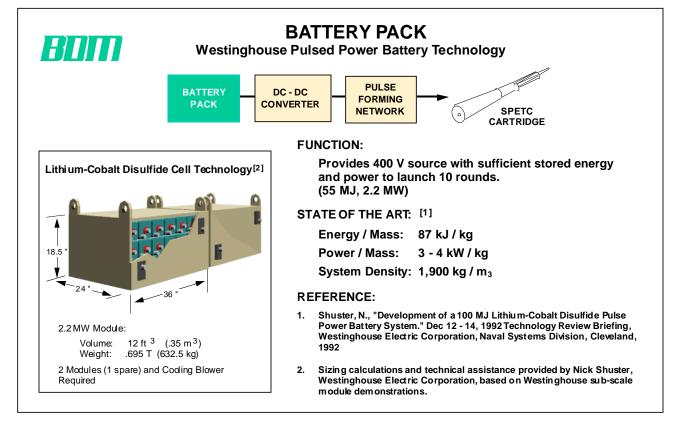
Figure 4: Technology Traceability Worksheet - Battery Pack Sizing
