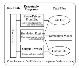
Figure 1: Components of a Special Purpose Simulator
