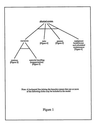
Presence of a station means that there are one or more identical servers which will be treated as the primary resource. Interpretation of the primary resource is up to the user. It may be a machine tool for a machining station, inspector for an inspection station, or simply a bench on which the assembly operation is carried out. The primary resource will be seized when a job arrives at the station, and released when it leaves.
