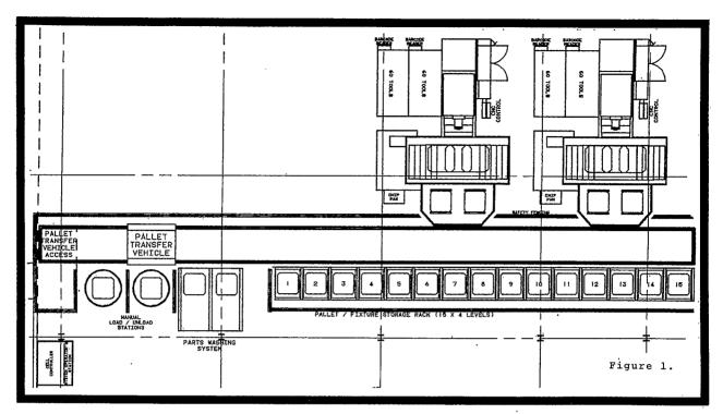
The parts washer has similar part handing capabilities to the machining centers previously described. Wash cycles are the same for all parts. Process duration is 3 minutes.
