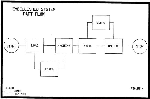
to storage as in the previous system. Figure 4 shows the revised material flow using a dashed line to represent conveyer travel and solid lines to represent crane travel.
