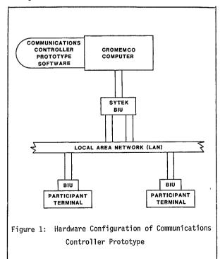
The Cromemco used for the prototype runs the CROMIX operating system, and the C-programming language is used for program implementation. An example of an exemplary message transmittal is provided in table 2.
