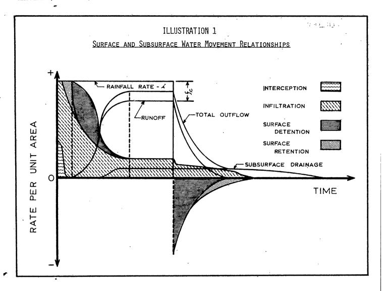
used in satisfying surface retention and detention. The difference between the inflow and outflow rates is integrated to provide a volume. When divided by the elemental area, this yields the average depth of water over an element. The depth, in turn, is used to determine an outflow rate by applying a runoff function that accounts for both runoff and detention.
