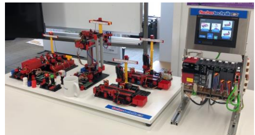
Figure 3: Advanced Production Twin model simulating a production line in the manufacturing process.
