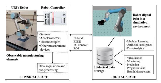
Figure 2: Data acquisition, usage, and exchange between the robot workcell and its digital twin.
