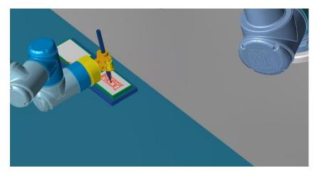
Figure 4: Simulation in a digital twin to help verify a robot program through visualization.
