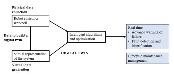
Figure 5: Role of data to support a PHM digital twin of a robot workcell.
