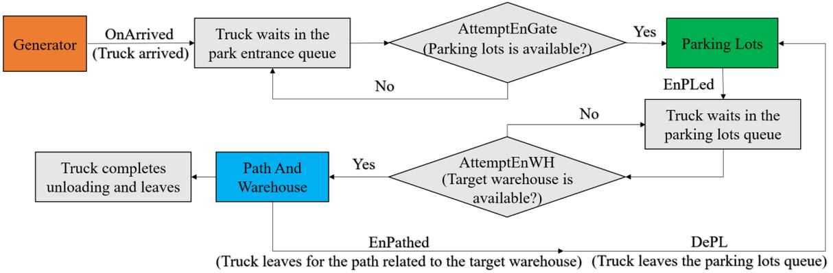
Figure 6: Logistics park simulation target model illustration.
