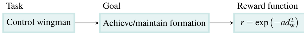
Figure 5: The task of the agent is to control the wingman aircraft, which amounts to achieving and maintaining formation, measured by a Gaussian reward function with a = 5 \cdot 10^{-7} \text{ m}^{-2} .
