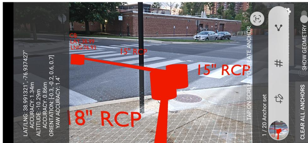
Figure 6: Superimposed utility layer on the real scene.
