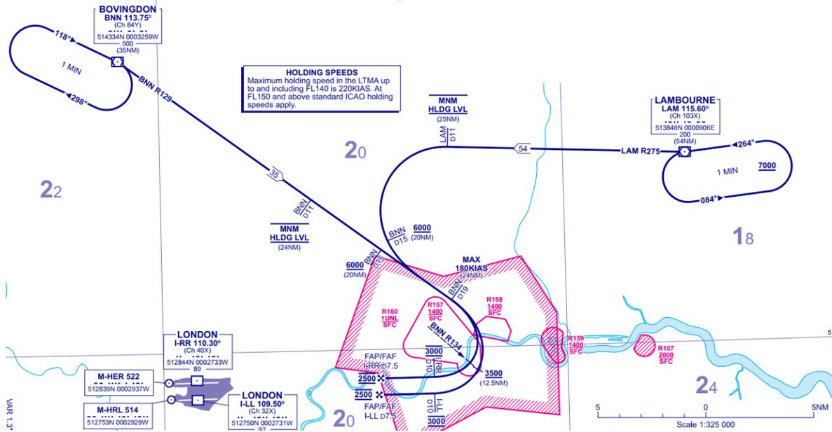
Figure 2: An aeronautical chart showing Bovington (left) and Lambourne (right), two of the four stacks that service London Heathrow, together with paths leading to FAFs for runways 27L and 27R.
