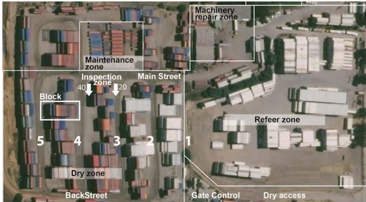
Figure 1 Layout of the Empty Container Depot
