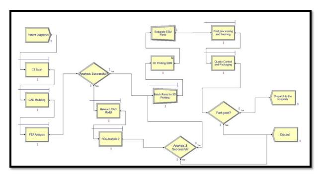
Figure 4 Simulation model for additive manufacturing of hip stems.
