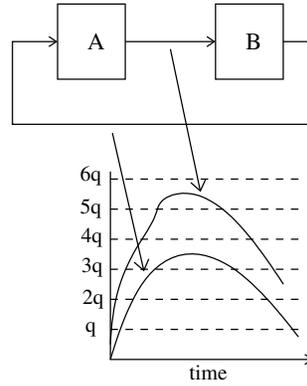
Figure 1: Two simulation components interacting via quantized output variables. New data for the continuous output variable is sent when it changes by a quantity  $q$ .
