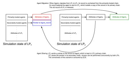
Figure 2: Cross state-enabled programming model for agent-based demographic models.
