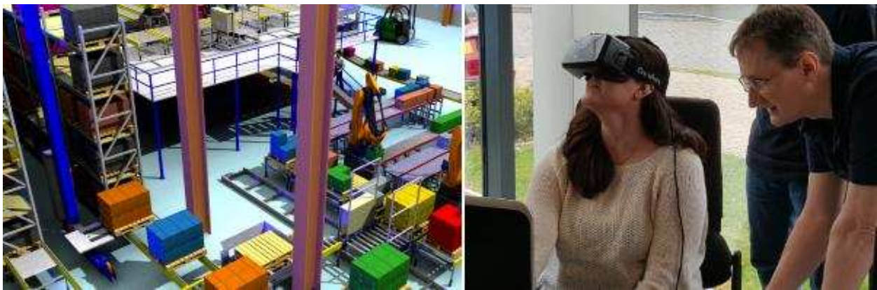
Figure 7: The Oculus Rift™ is just one way users can view Emulate3D models in stereo 3D
