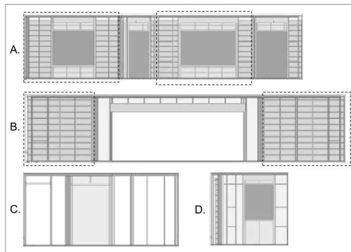
Figure 2: Multi-wall panel: (A) Exterior multi-wall panel with windows and doors; (B) Garage wall with garage door; (C) Interior multi-wall; (D) Short exterior multi-wall.
