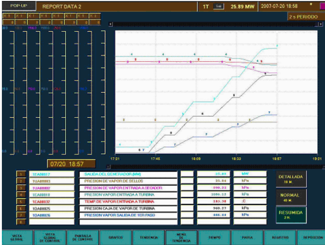
Figure 4. Cerro Prieto-IV Simulator . Manual power plant Start-Up
