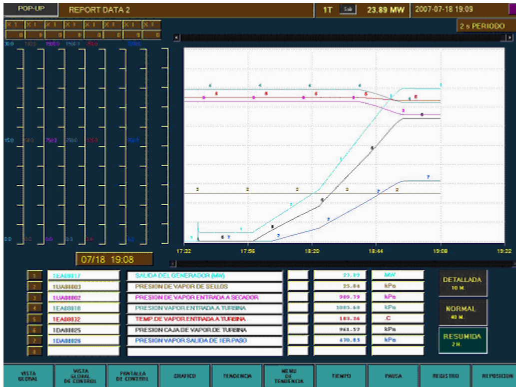
Figure 5. Simulator of Cerro Prieto IV, Automatic Start-Up of the power plant
