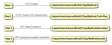
Figure 10: DCD++ Steps by a Client Example
