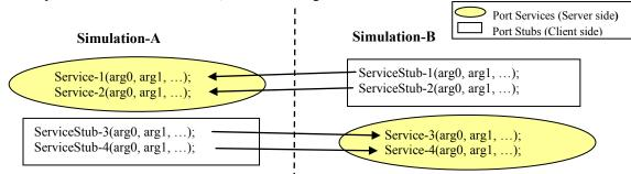
Figure 1: SOAP-based Web-services RPC-based Programming Model
