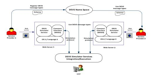
Figure 3: Overall system of interoperable DEVS simulator services
