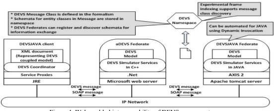
Figure 4: Web-enabled interoperability of DEVS components
