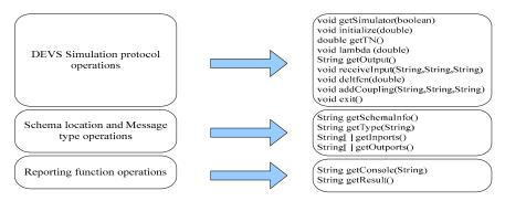
Figure 6: The operations of DEVS simulator service
