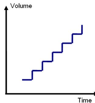
Figure 3: Discrete representation of the material arriving at the destination point (modeled system)
