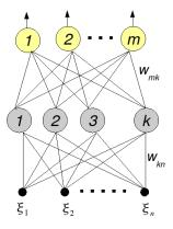
Figure 1: Structure of a Typical Multi Layer Perceptron with One Hidden Layer with k Units
