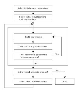
Figure 6: Sequential Design with Adaptive Modeling
