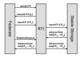
Figure 2: Check-Pointing Mechanism in the DRMS.
