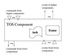
Figure 1: Structure of a TinyOS Component
