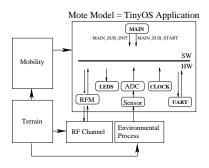
Figure 4: Architecture of the TinyOS Scalable Simulation Framework
