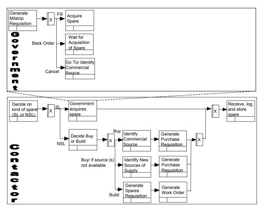
Figure 4: PROSIM Simulation Model Design for the Spares Acquisition Supply Chain Process
