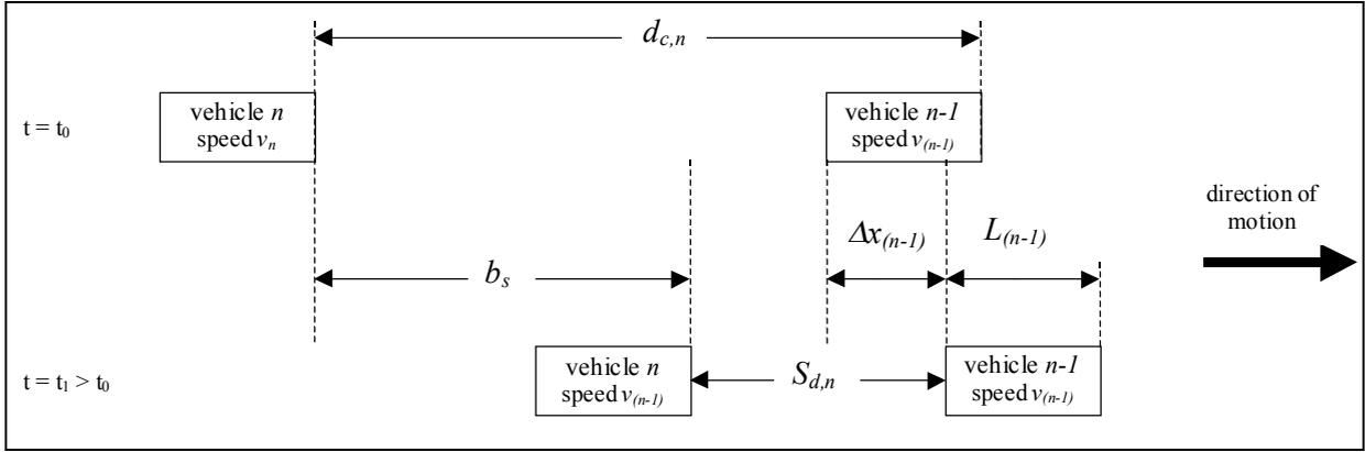
Figure 2: Critical Distance for Vehicle  $n$
